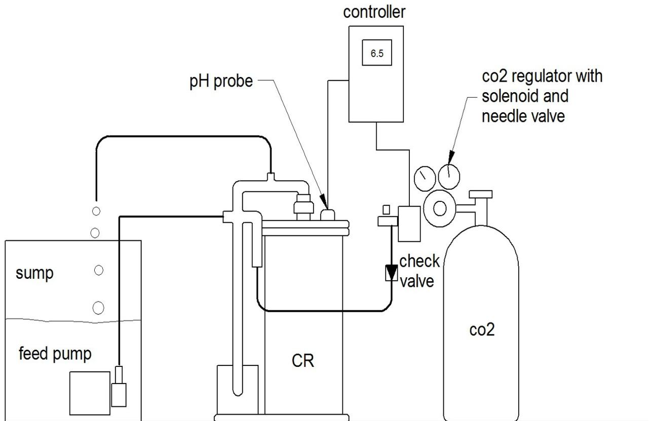
**This is a diagram of a typical calcium reactor installation. The cobalt MJ (or other) feed pump draws water from the display sump and pumps it into the calcium reactor. Water is mixed with co2 circulated through the calcium carbonate media in the chamber and then allowed to flow back into the sump.**
